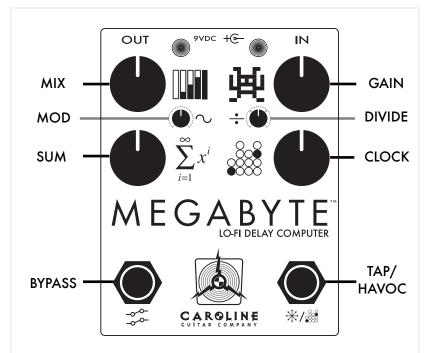
A lot is happening here, and it all still fits on a card! The GAIN sets the input drive of the delay preamp. The binary CLOCK sets the delay time. SUM is the number of repeats. MOD introduces a subtle variation in the delay time that can be dialed up to create a chorus or detuned effect to the repeats. The MIX control is the overall volume of the \*wet\* signal. The more gain you add, the lower this will need to be for unity with your clean signal.
