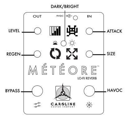
ATTACK sets the amount of gain in the preamp, allowing you to boost or overdrive the reverb. SIZE establishes the initial reverberation.
