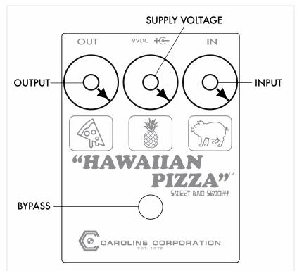
Be sure to take your thinking caps \*off\* for this one. INPUT (pig) controls your instrument's feed to the transistor amplifier. Full on is full-blast, dial it back for crunch. VOLTAGE (pineapple) is the power supply to the amplifier circuit. Turn it up for max headroom, back it off for squishy compression, or way down for fun broken, gated, & octave-y sounds. OUTPUT (pizza) is the final output level. The more of the other controls, the less you'll need of this. And vice versa.
