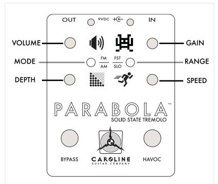
GAIN controls the first preamp stage; for cleaner sounds, leave this set low (though what fun is that?). SPEED and RANGE set the Tremolo LFO rate. DEPTH affects the intensity of the effect and the shape of the waveform. VOLUME is the overall output after the second preamp stage. It can get LOUD.
