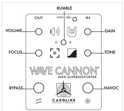
GAIN controls the amount of distortion. TONE makes the output brighter or darker. FOCUS scoops, flattens, or boosts the midrange frequencies. VOLUME controls the overall output. RUMBLE increases the amount of bass available in the circuit, and is especially useful at lower gain settings. Flipping this switch may cut your signal momentarily; this is perfectly normal.
